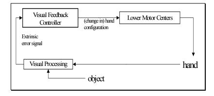
Figure 7.6 The schema level view of the feedback controller. The visual processing encapsulates the process of extracting an error based on the vision of the hand and the object. Lower Motor Centers encapsulates the functionality involved in transforming the motor signal into actual commands sent to muscles
