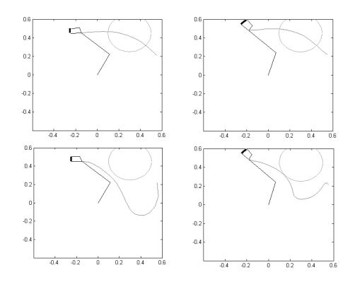
Figure 7.15 The top row demonstrates two trajectory-planning examples for grasping without obstacle. The bottom row demonstrates how new trajectories are formed by introduction of an obstacle as a local inhibition on the feed-forward controller units
