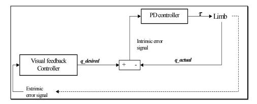
Figure 7.9.The Visual feedback circuit generating desired trajectories for the 'lower level motor centre' (implemented as a PD controller)
