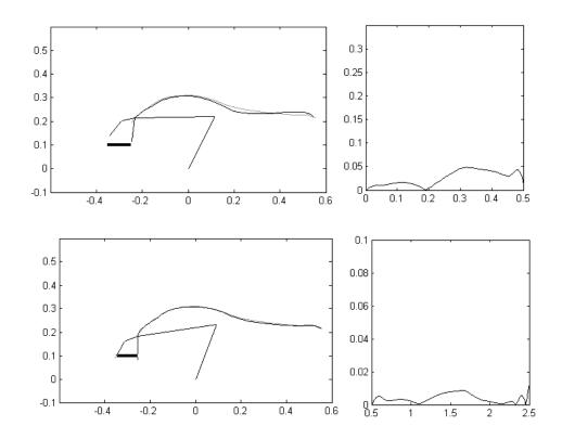
Figure 7.14 The feedback, feed-forward and lower level motor servo and the dynamic arm was simulated all together. Upper half: The grasp lasted 0.5 seconds. Lower half: the grasp lasted 2 seconds. The fast movement error reduced with a factor of 6 while the slow movement reduced with a factor of 10 in terms (compare with Figure 7.10)
