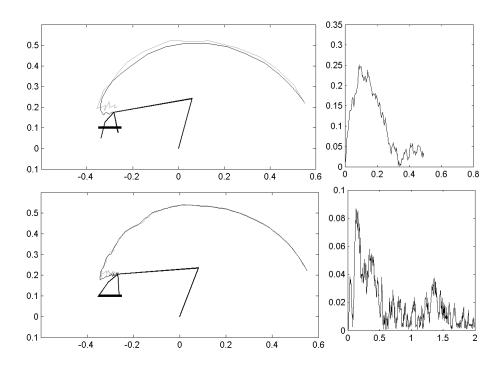
Figure 7.10 The slow (2 seconds) (lower half) and fast (0.5 seconds) (upper half) performance of the 'visual feedback servo' + 'PD controller' system is shown. The right hand side graphs show the tracking error (of the wrist) versus time. In the slow case, the object can be grasped but in the fast case, it is missed
