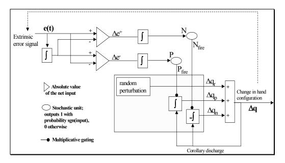
Figure 7.7 The leaky integrator implementation of the feedback circuit that solves the inverse kinematics problem for precision grasping. See text for the explanation
