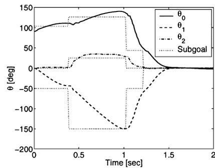
Fig. 14. Example of a time course of a stand-up trajectory and a sub-goal sequence ( $\theta_0$ : pitch angle,  $\theta_1, \theta_2$ : joint angle).
