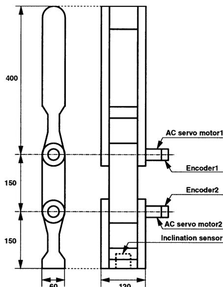
Fig. 11. Real robot configuration.
