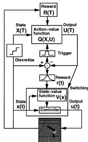
Fig. 2. Hierarchical reinforcement learning architecture.
