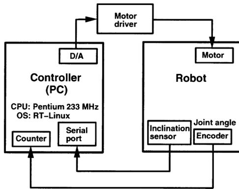
Fig. 12. System configuration.
