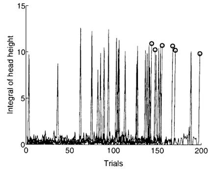
Fig. 13. Time course of learning with real robot. Circles show 10th successful stand-up, upon which a simulation run was terminated.
