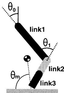
Fig. 6. One-joint, two-link robot configuration.
