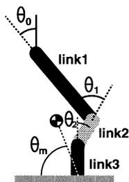
Fig. 1. Robot configuration.  $\theta_0$ : pitch angle,  $\theta_1$ : hip joint angle,  $\theta_2$ : knee joint angle,  $\theta_m$ : the angle of the line from the center of mass to the center of the foot.
