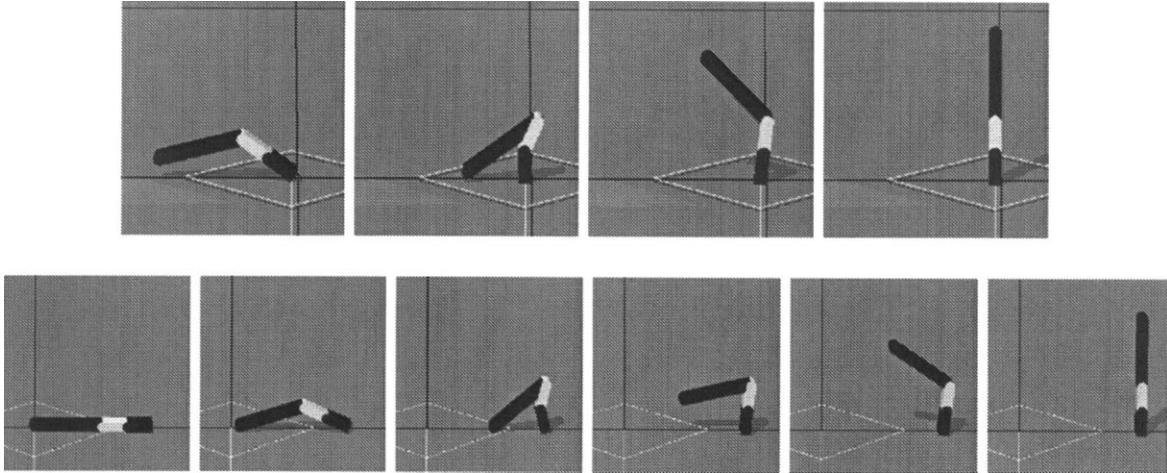
Fig. 5. Example of a successful sub-goal sequence (top); example of a successful stand-up trajectory (bottom).
