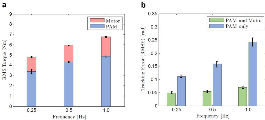
**Fig. 8.** Torque distribution: (a) contributions of each actuator to generate joint torques. Contribution of electric motor was much smaller than that of PAM in terms of amount of generated torque; (b) tracking errors of proposed hybrid control method and PAM-only approach. Results clearly indicated that electric motor greatly improved tracking performances, even though amount of output torque was much smaller than that of PAM.
