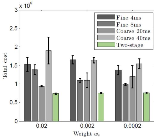
**Fig. 4.** Control performances with three different weights of voltage input cost:  $w_v = 0.02, 0.002$  and  $0.0002$ . Accumulated costs for 10-s duration of five tracking control trials were compared. We utilized the target trajectory with frequency of 1.0 Hz. Our proposed approach showed best control performance regardless of weight settings. Error bars represent standard deviations.
