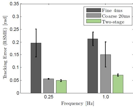
**Fig. 6.** Averaged tracking errors of five experimental trials each of the fine, coarse and proposed strategies. We found that our proposed approach outperformed the standard MPC implementations. Error bars represent standard deviations.
