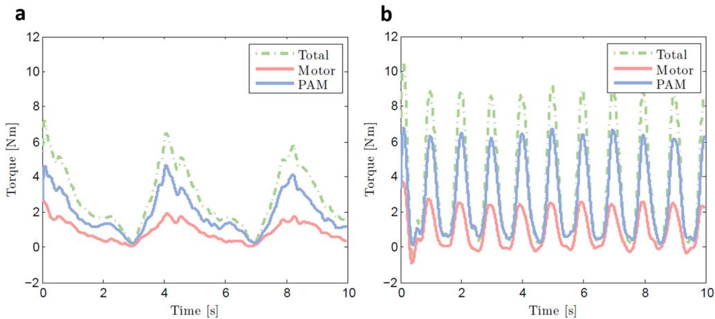
**Fig. 9.** Generated joint torque profiles to present how torque was dynamically distributed to each actuator for target sinusoidal trajectories of 0.25- and 1.0-Hz frequencies. For both target frequencies, PAM and electric motor were cooperatively activated for target tracking tasks. Moreover, the electric motor sometimes acted like antagonistic muscle in both cases for precise tracking by properly generating force to oppose direction of force generated by PAM.
