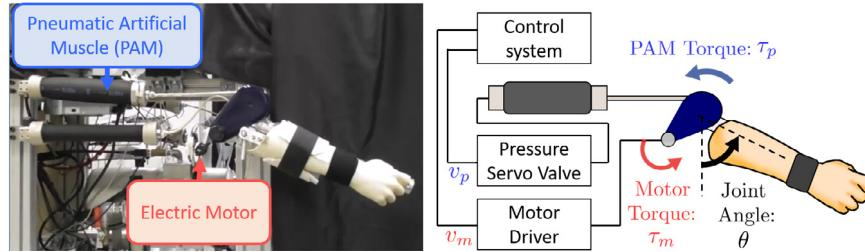
**Fig. 1.** Forearm robot with pneumatic–electric hybrid actuator system: pneumatic artificial muscle dominantly generates torques but is assisted by small and lightweight electric motor for precise movements.  $v_p$  denotes voltage input for air valve, and  $v_m$  denotes voltage input for motor driver. We used one pneumatic artificial muscle and one electric motor.
