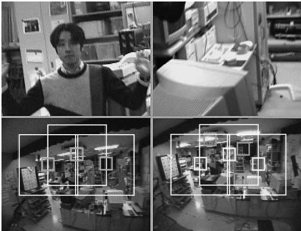
Figure 19: VOR-OKR learning with three template trackers: the monitor output of four cameras (two eyes) are shown. The bottom half images show the peripheral vision output where there are three large white rectangles showing search areas and three small rectangles showing the current target positions.
