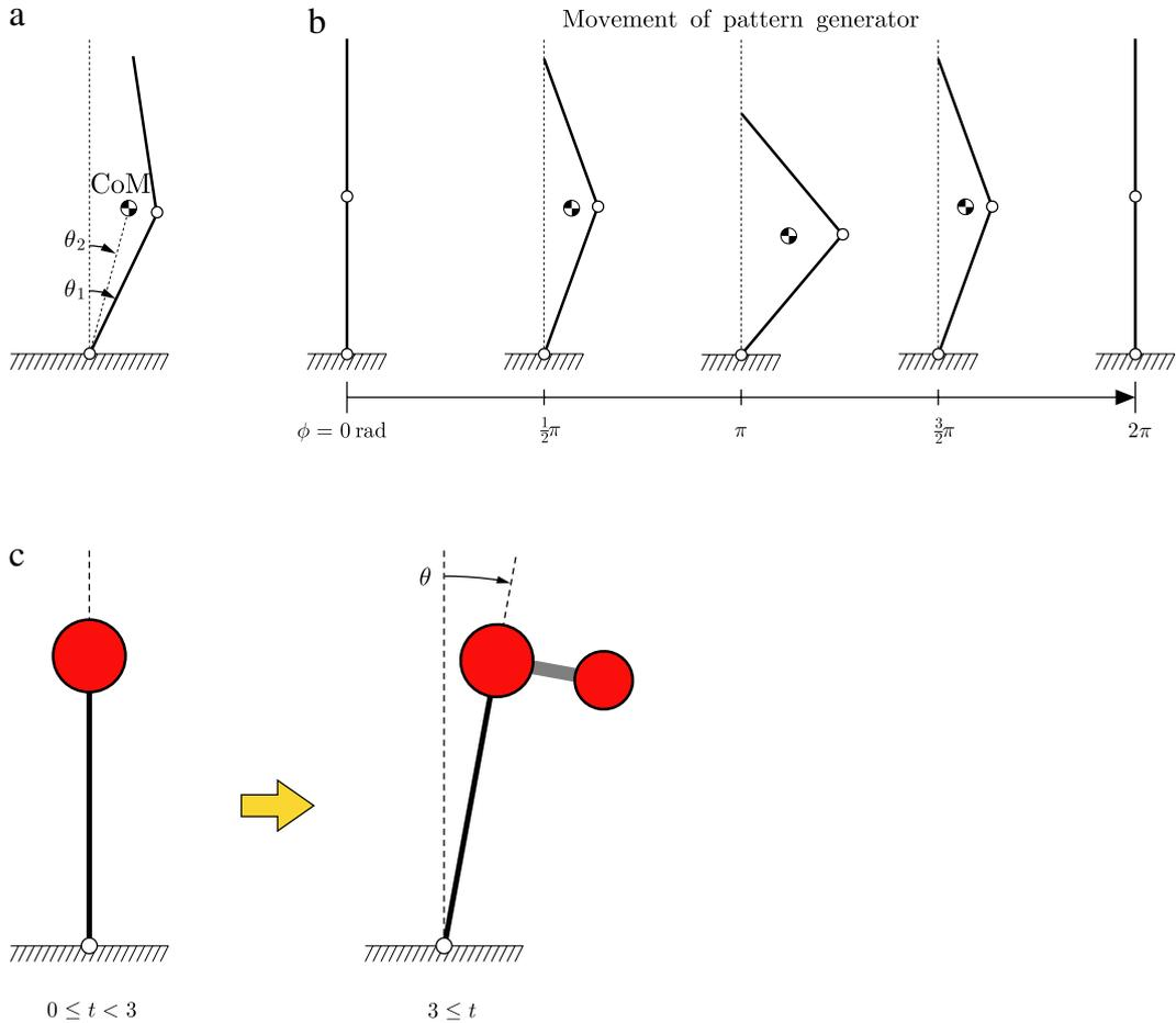
**Fig. 3.** (a) Two-link robot model. The mass and length of each link are 5 kg and 0.5 m, respectively, and the friction coefficient of each joint is 0.1. (b) Relationship between the phase of the periodic pattern generator  $\phi$  and the posture of the two-link robot model. For details, see Appendix D. (c) Single pendulum model with payload. The masses of weights attaches at the corner and tip are 10 kg and 5 kg, and the lengths of long and short axes are 1.5 m and 0.5 m, respectively.
