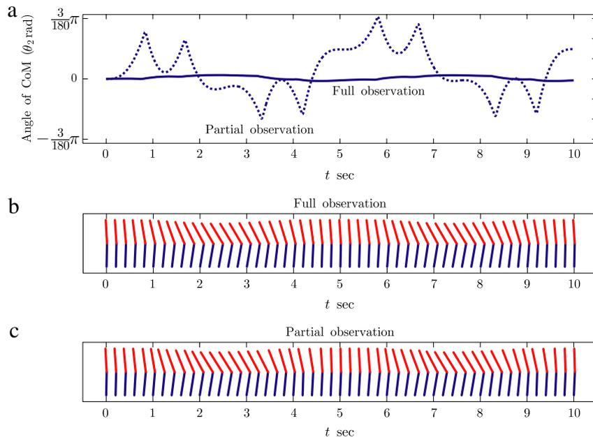
**Fig. 6.** Results of squatting task in full observation and partial observation environments. (a) Trajectory of CoM ( $\theta_2$ ). The solid and dashed lines represent full and partial observation cases, respectively. (b), (c) Squatting movements of full and partial observation cases (see *Movie 1*).
