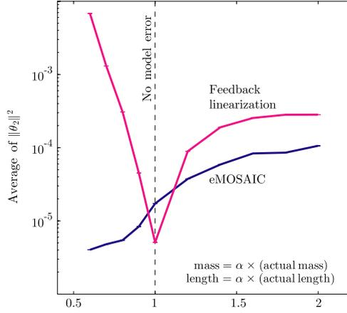
Fig. 7. Results of robustness test of eMOSAIC and feedback linearization. The horizontal axis is the parameter  $\alpha$  defining a modeling error. The vertical axis is the angle of CoM ( $\theta_2$ ). The mean and standard deviation of 50 trials are plotted.
