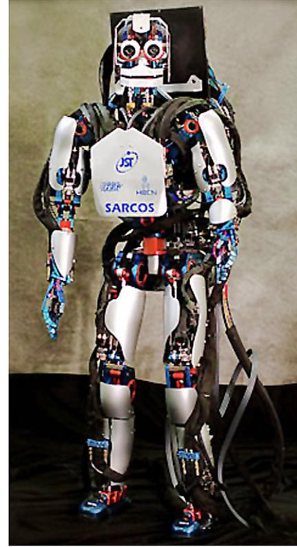
**Fig. 1.** Humanoid robot CB-i. Height: 1.6 m. Weight: 90 kg. Robot has 51 degrees of freedom.
