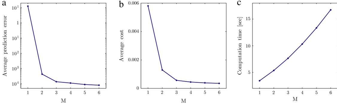
**Fig. 4.** Evaluation result of (a) average prediction error, (b) average cost, and (c) computation time for different number of modules, respectively.
