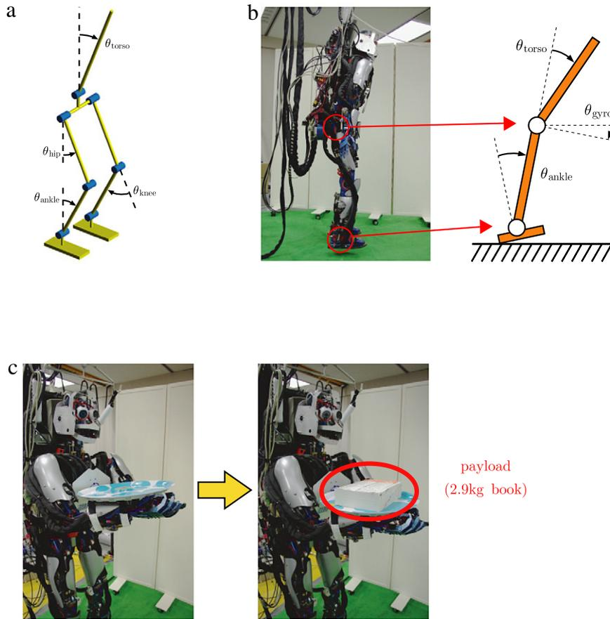
**Fig. 9.** (a) Joint coordinates of humanoid robot CB-i. (b) Two-link robot with foot model of the CB-i. The two joints of the two-link model represent the torso and ankle joint of the CB-i. The gyro sensor is attached to its hip. (c) Lifting task. Payload mass is 2.9 kg. Left: without payload. Right: with payload.
