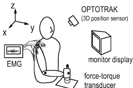
Fig. 2. Schematic drawing of the experimental setup
