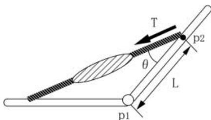
Fig. 1. Model of a mono-axis joint
