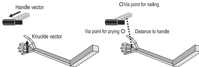
Fig. 10. The control variables used in nailing and prying tasks are depicted. The desired Knuckle vector is  $-(\text{Handle vector})$  for prying and  $(\text{Handle vector})$  for nailing. The desired Distance for both cases is zero. The path of the hand is constrained with appropriate via-points to avoid collision.
