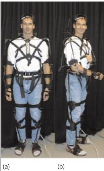
Figure 12. The Sensuit motion-capture system.
