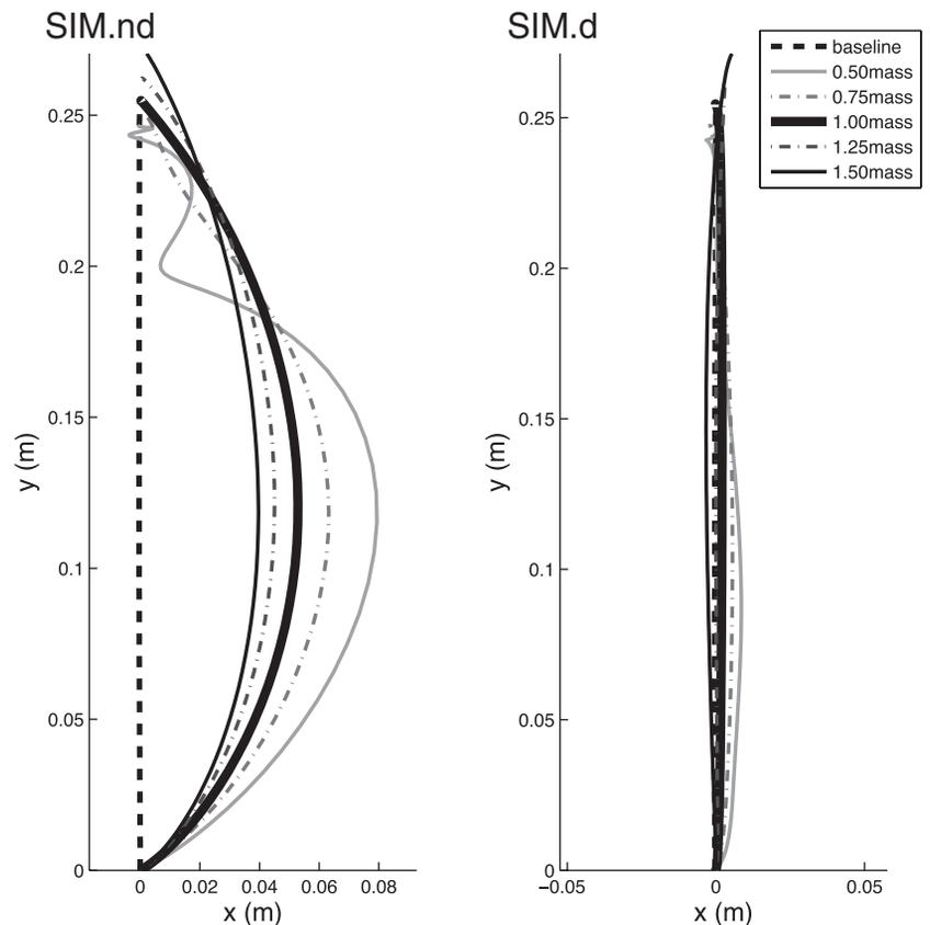
Fig. 8. Sensitivity of the controller with respect to unknown changes in arm mass. In each case, the optimal controller is computed assuming the nominal mass value, but tested on 50, 75, 100, 125, and 150% of the mass value. SIM.nd uses the nondirectional cost function, and SIM.d uses directional cost.
