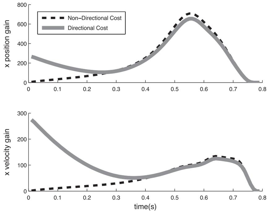
Fig. 7. Position and velocity gains of the optimal controller, in the  $x$  direction (same direction as the force perturbation) before and after addition of a directional constraint to the cost function. Adding the directional constraint effectively increases stiffness and damping during the early part of the movement.
