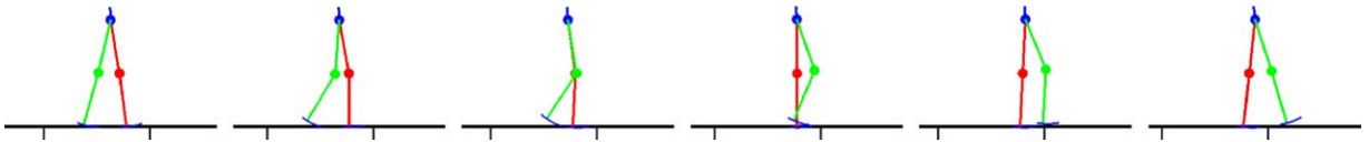
Fig. 4. Snapshots of walking simulation for one step at 15 frames/s (1 frame \approx 66 ms).
