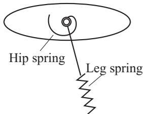
**Figure 1:** *Passive one-legged hopper*
