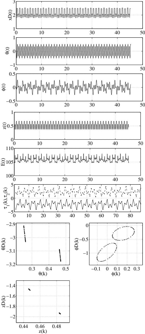
**Figure 3:** Simulation result of “Non-Dissipative Touch-Down Control”. The lower four small graphs represent the selected images of the Poincaré map. From this, you can see the gait obtained is quasi-periodic one.
