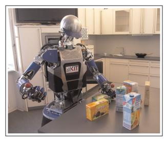
**Figure 3.** The humanoid robot ARMAR-III interactively discovers objects that can typically be found in a kitchen environment, segments them and learns their visual appearance.
