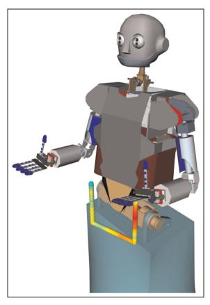
**Figure 5.** Reachability values on a pushing path for the left hand of ARMAR-III. Dark red dots indicate low, bright yellow dots high reachability values.
