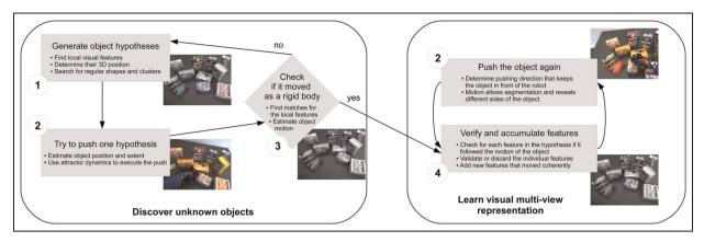
Figure 1. A diagram showing the general structure of our approach to discovering new objects and learning their appearance.
